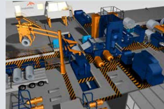
▲ Stand-alone temper mill for automotive applications at ArcelorMittal Dofasco
