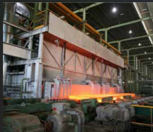
▲ Double regenerative burners for largest European HSM furnace
