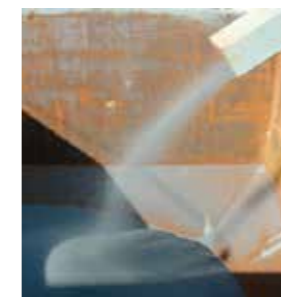
▲ High-density Oxide produced by Fluidized Bed ARP
