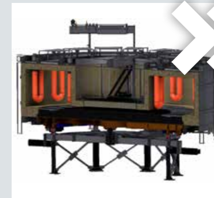
▲ Rotary Hearth Furnace
