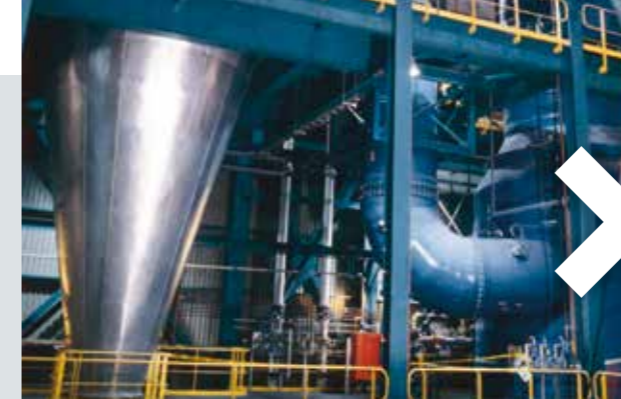
▲ Spray Roaster Pyrohydrolysis for nickel oxide extraction Goro Nickel, New Caledonia
