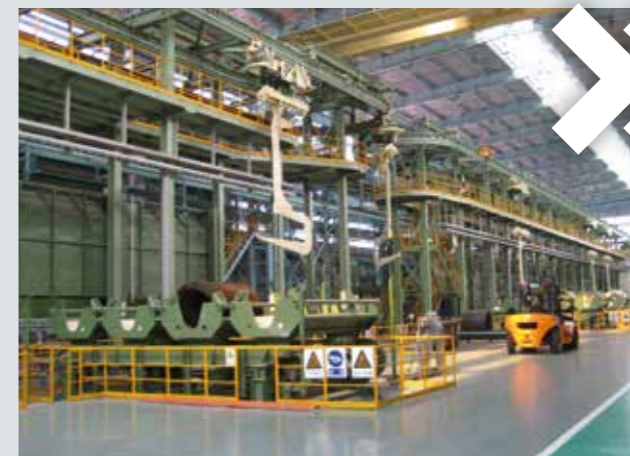
▼ Fully automated Wire Coil Pickling Line with Salt Bath for Baosteel, China
