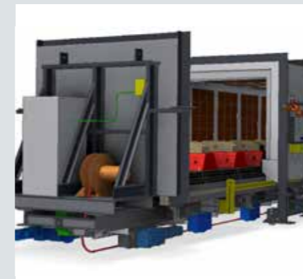
▲ Car Bottom Furnace with Electric Heating Elements
