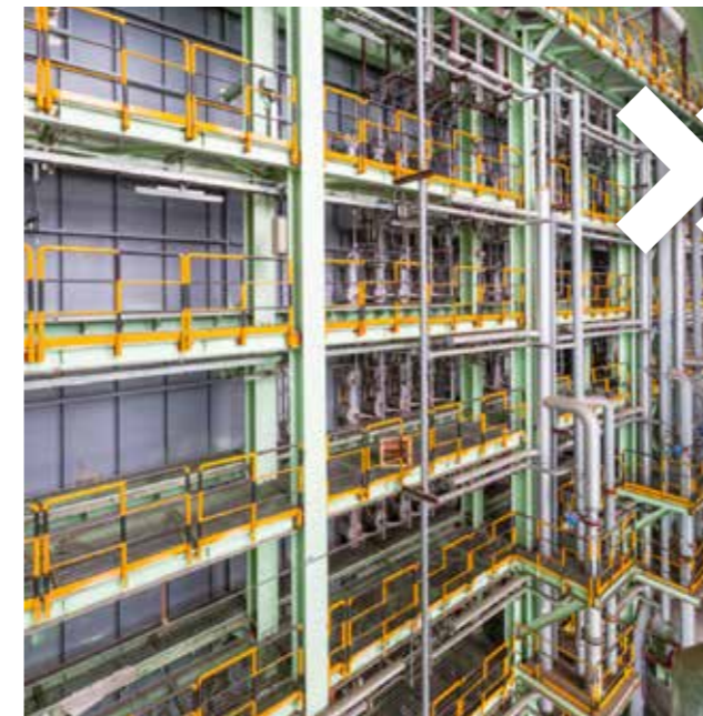
▲ Vertical line furnace on CAL, Shagang, China
